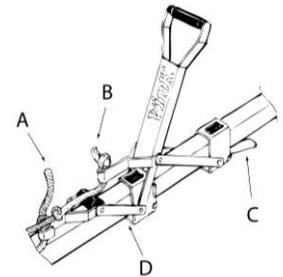
The lever mechanism of the VINK calfpuller with alternate traction is equipped with 2 hooks which will be drawn backwards one by one when pulling the handle backwards. The distance between the two hooks when pulling is approximate 7 cm. The distance between the knots in the ropes must be the same to ensure equal traction on both legs of the calf.
